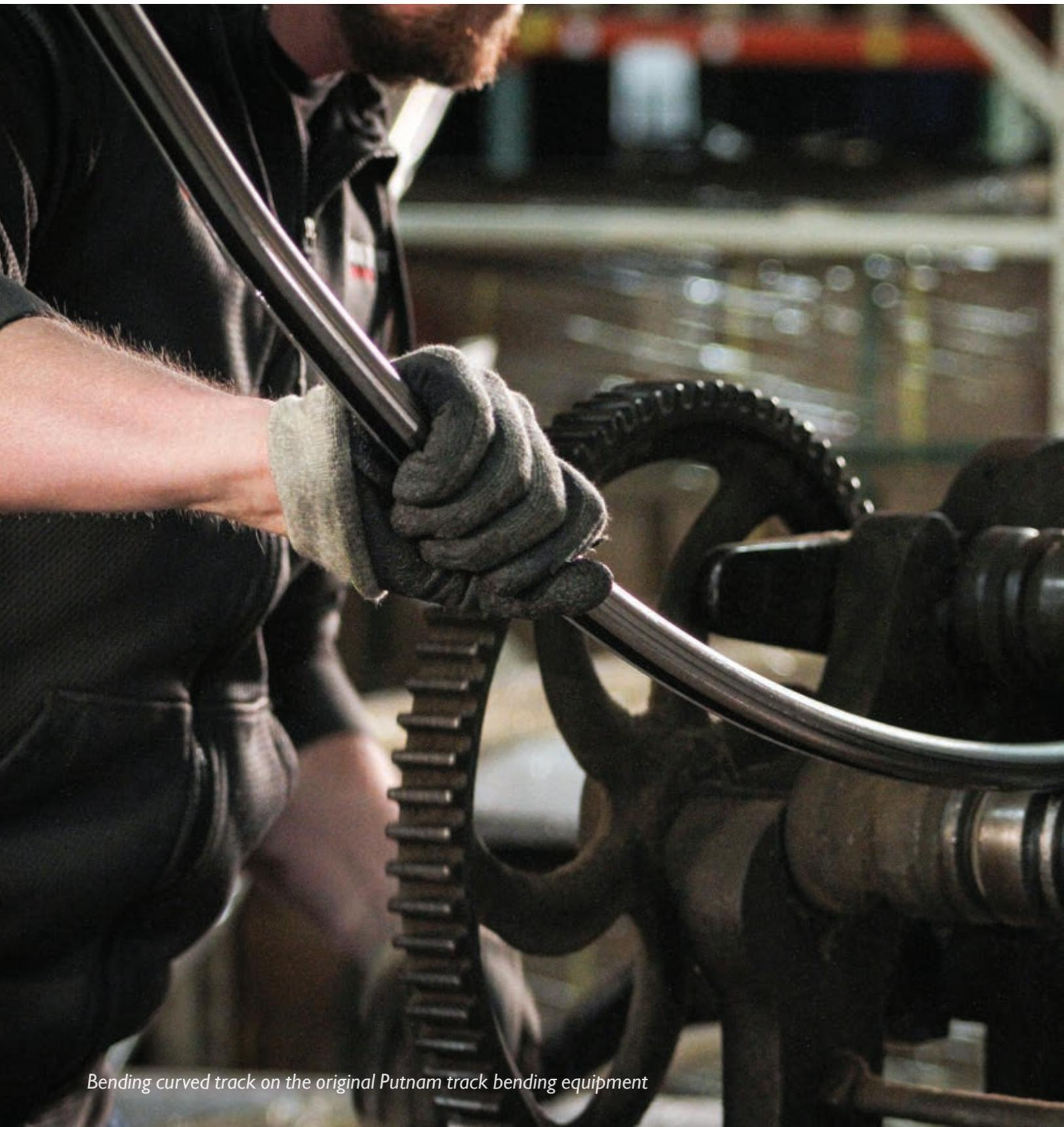
*Bending curved track on the original Putnam track bending equipment*
