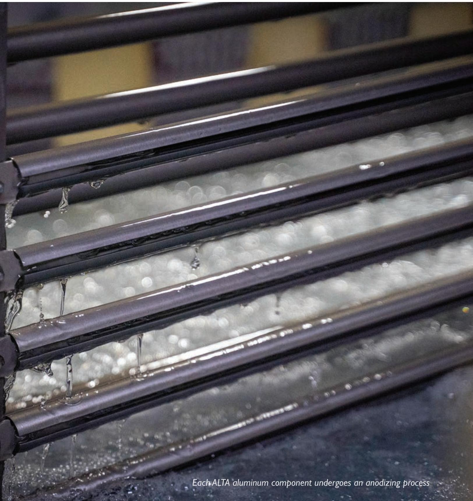
*Each ALTA aluminum component undergoes an anodizing process*
