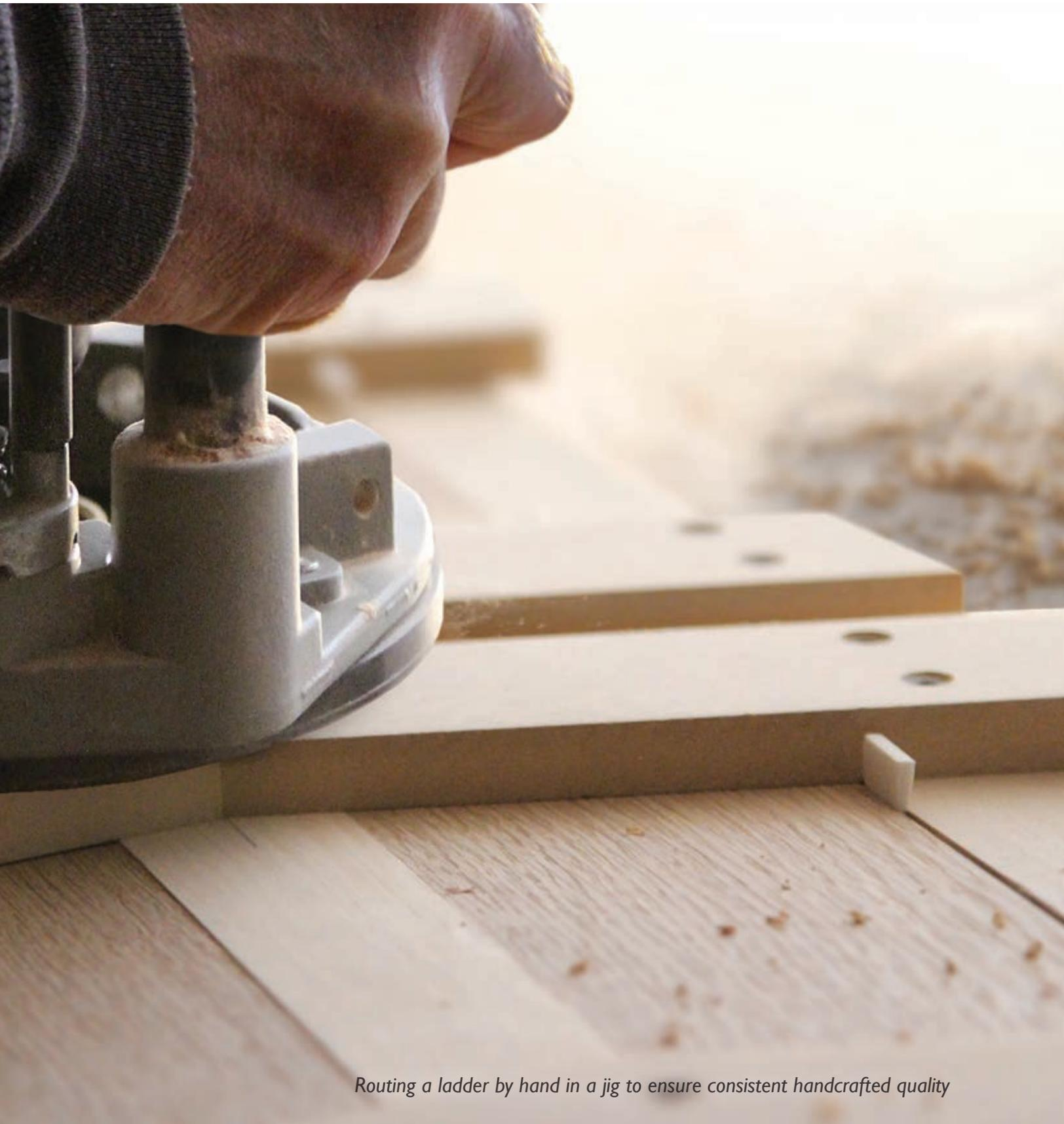
*Routing a ladder by hand in a jig to ensure consistent handcrafted quality*
