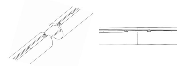
3. Slide all the track mounting brackets onto the track, leaving them loose on the track. Brackets should be spaced no further than 32" apart and 8" from each end.
